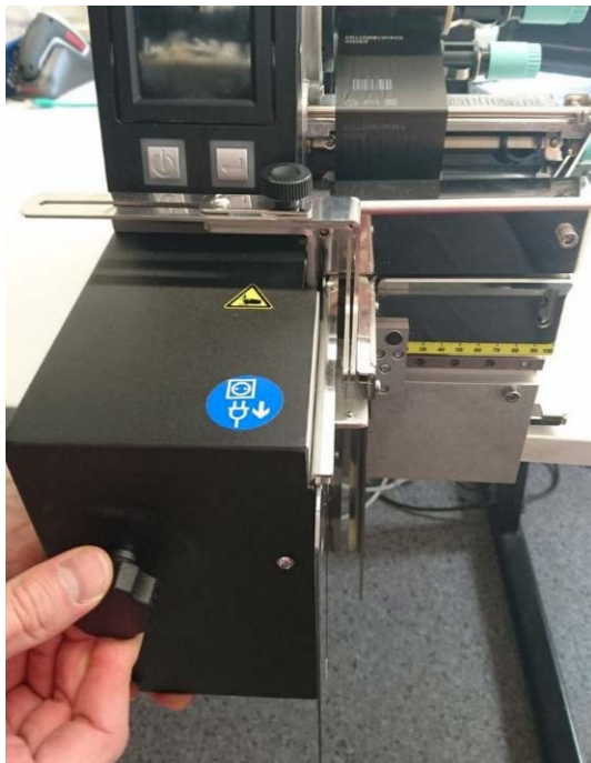
Pic. 8. Support the Cutter Stacker with one hand and tighten the screw with your free hand.
